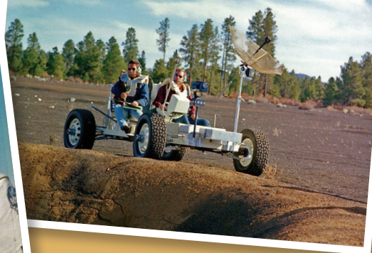
Astronauts Jim Irwin and Dave Scott test lunar rover vehicle simulator "Grover" in Cinder Lake Crater Field, 1970 (photo: NASA)
