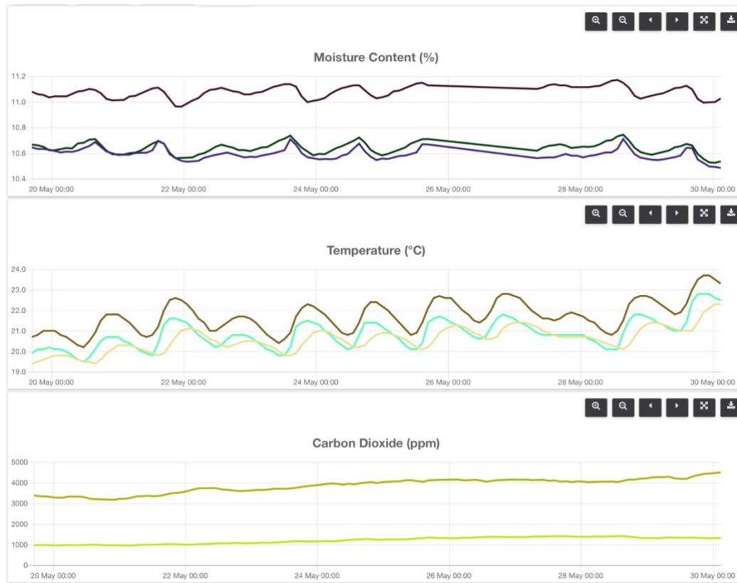
Figure 2: Monitoring of conditions with sensors in grain (available at centaur.ag )
