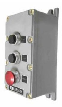
The Larson Electronics EPCS-2XMPB-1XEST-MOD1 Explosion Proof Control Station is suitable for busy operations in hazardous locations. Featuring five drilled and tapped operator holes, the unit supports several control mechanisms for heavy-duty machines. One emergency stop pushbutton and two momentary jog pushbuttons can be found on this station. Constructed of aluminum with stainless steel components, the NEMA-rated unit is surface mount compatible.
