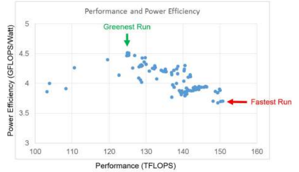
Fig. 8. Results of Linpack benchmark runs with various configurations. Each dot corresponds to a single Linpack run.
