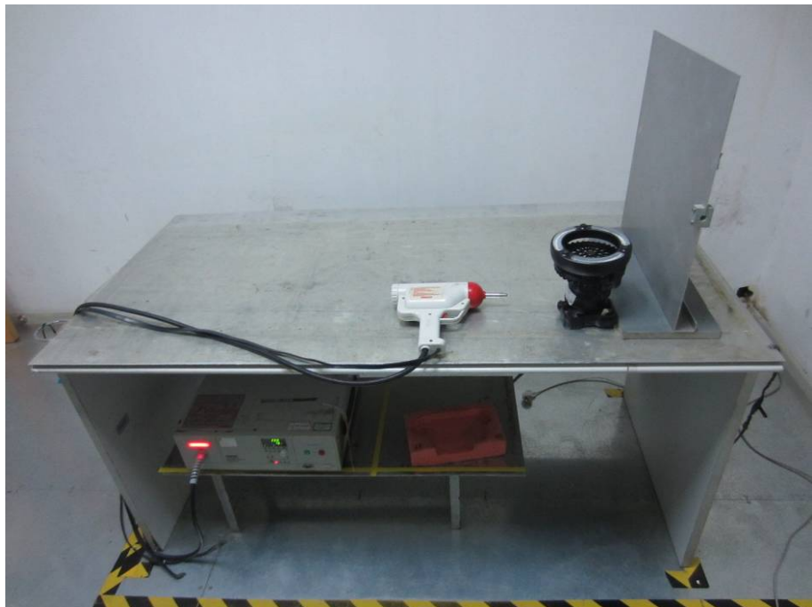
ESD Test Setup Photograph
